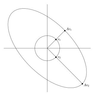
**Figure 2.1.1.** Behavior of the linear transformation A in (2.1.8), with two distinct real eigenvalues
